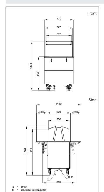
Electric Supply voltage: 220-240 V/1N ph/50 Hz Electrical power, max: 0.49 kW Capacity: Capacity - nr./plates: 0 **Key Information:** N° of doors: External dimensions, Width: 770 mm 1180 mm External dimensions, Depth: External dimensions, Height: 1304 mm Net weight: 108.5 kg Shipping height: 1334 mm Shipping width: 810 mm Shipping depth: 899 mm 0.97 m<sup>3</sup> Shipping volume: -10 / 0 °C Set temperature: -10 / 0 °C Top temperature:
